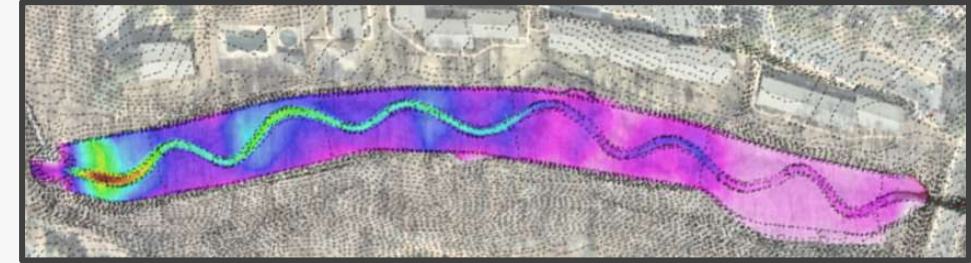
Design Option 1 Bank Shear Analysis
