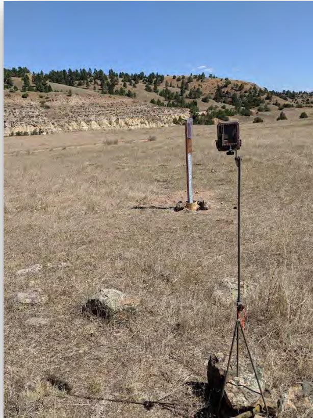
3 camera trap precip gages
